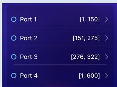
In the above example, the first output controls all the lights for the lower section of the building. That output has light 1 through light 150. The 2nd output which is the upper story of the project has light 151 through light 275.
